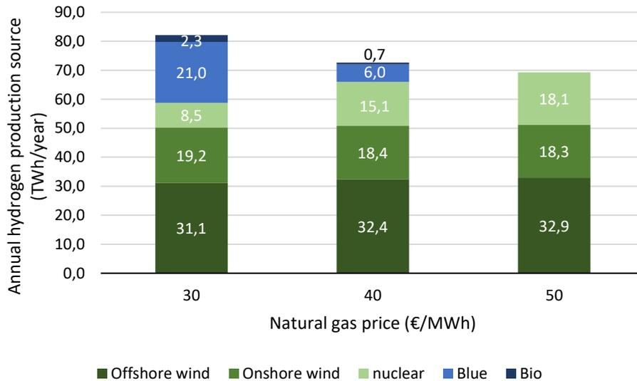
Figure 9. Sensitivity of the hydrogen supply mix and demand to the natural gas price
