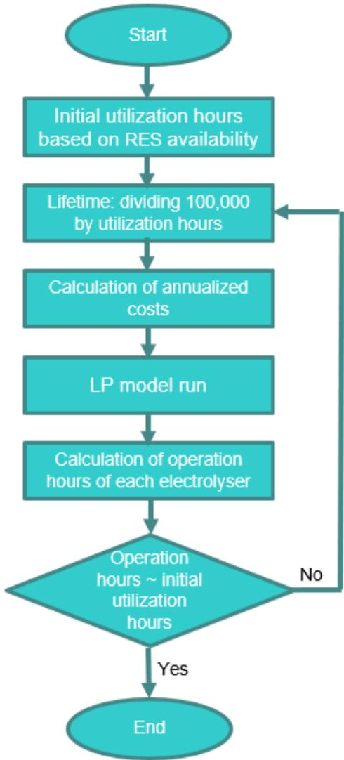
Figure 2. Iterative methodology of electrolyzer lifetime calculation
