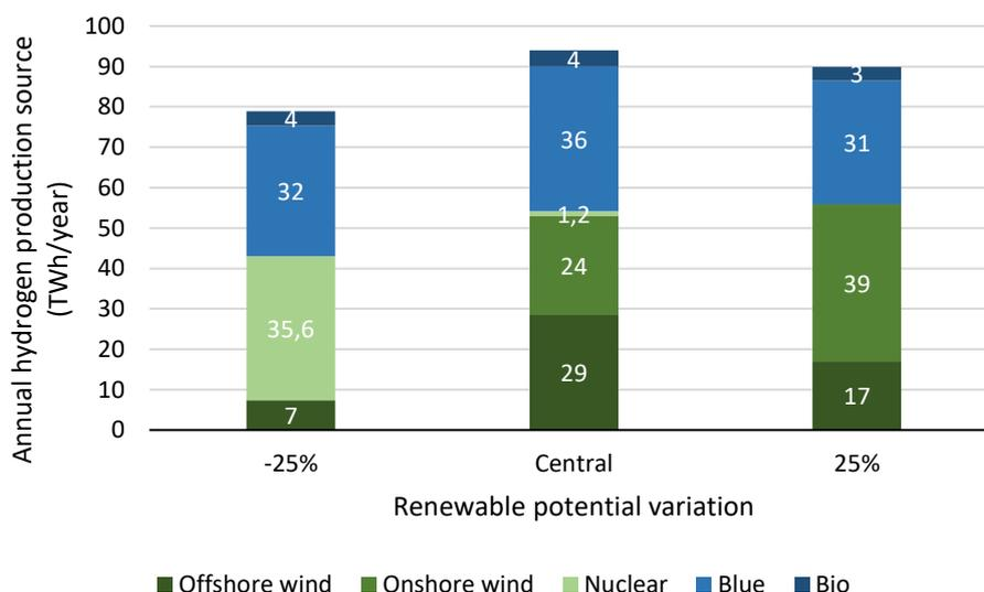
Figure 7. Sensitivity of the hydrogen supply mix and demand to renewable potential
